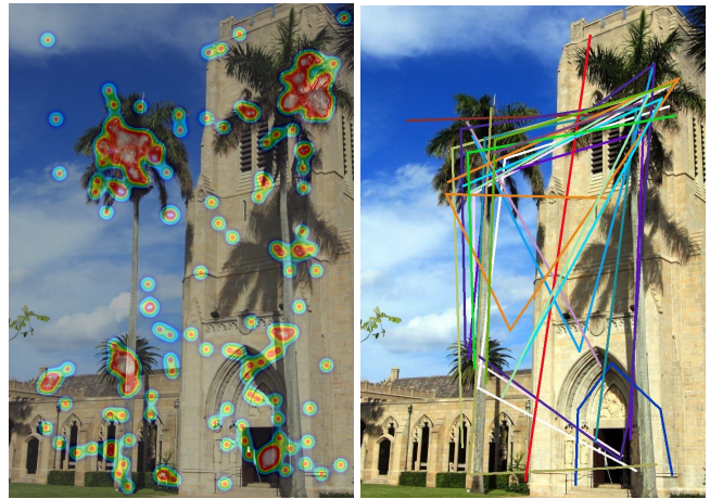
Figure 1. Image-based passwords consist of a series of passwords defined on an image (left). Hotspots, i.e., popular features of the image that are frequently selected, may compromise security (right).
