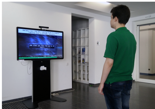
Figure 4. Trivia Game: Answers to questions are provided in the form of images. Only as users approach the sweet spot they can see the unmodified image and hence the answer to the question. As users remain in the sweet spot for some time we also display a textual answer before switching to the next question.
