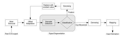
Fig. 1. Artefact Compensation Framework Flowchart
