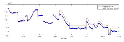
Fig. 2. ACF corrected EOG signal
