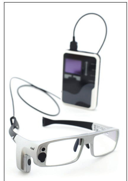
Figure 2. Tobii Glasses. This recently released video-based eye tracker is the first system to fully integrate into an ordinary glasses frame (photo courtesy of Tobii Technology).
