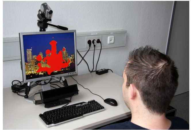
Figure 4: Experimental setup used in the pre-study. Participants selected image-based passwords, gazing at images with and without a saliency mask, as well as PINs on a standard 10-key keypad. Gazes were recorded using a remote eye tracker placed under, as well as a high-resolution video camera mounted above the computer screen.
