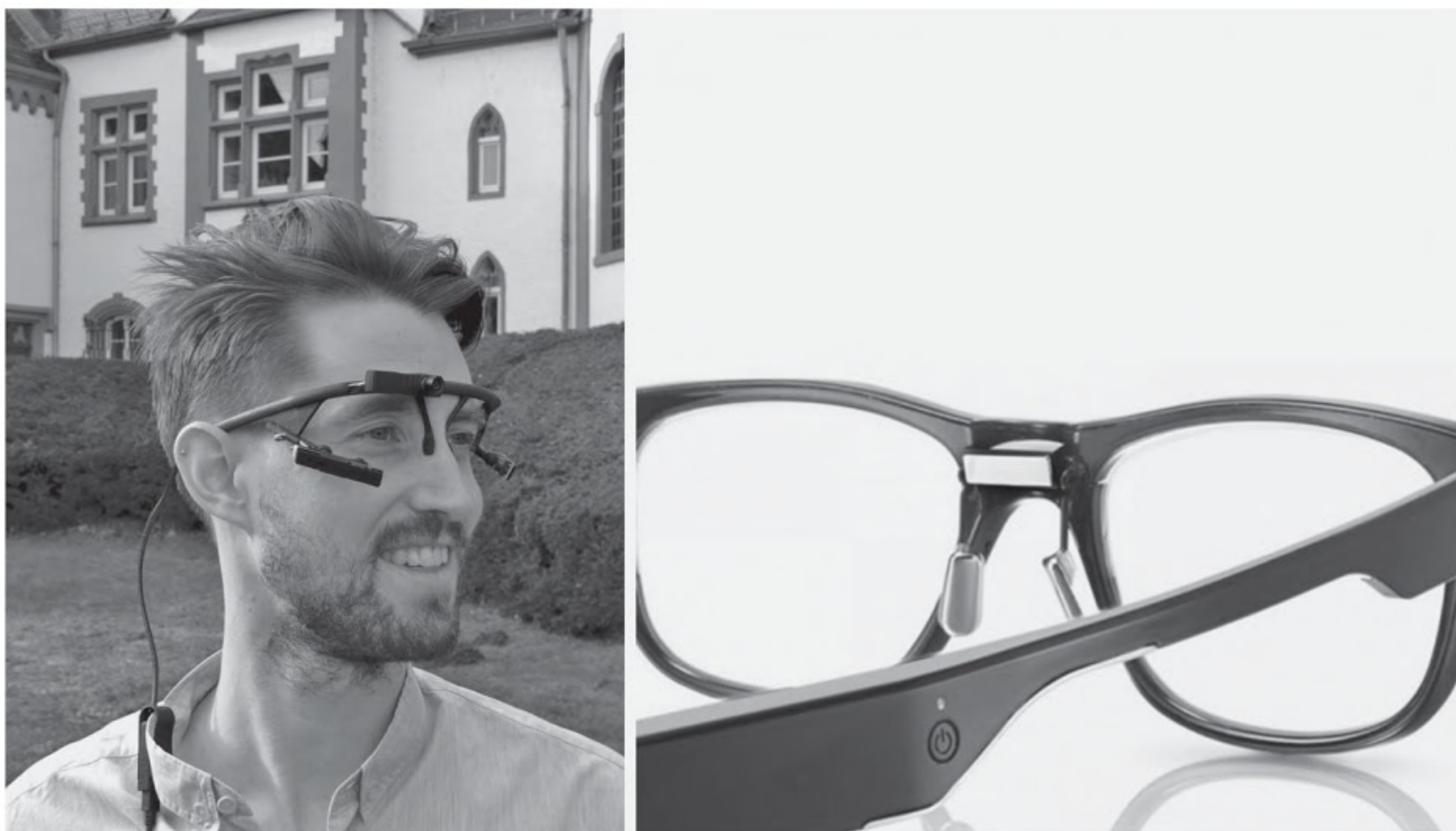
FIGURE 2.1 (left) PUPIL from Pupil Labs is an accessible, affordable, and extensible open source platform for mobile eye-tracking, gaze-based interaction, and egocentric vision research. (right) MEME from J!NS is an integrated eyewear computer for measuring eye movements using Electrooculography (EOG) and head movements using integrated inertial sensors.
