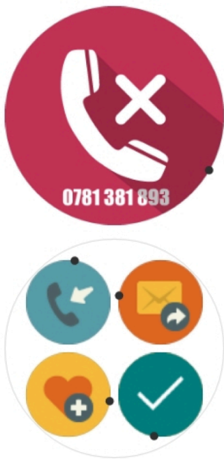
Figure 4: The missed call menu interface. Top: an Orbit control with an iconic representation informing the user of a missed call. Upon following the target the user is shown four other Orbits, each with an iconic representation of an action: call back, text back, add to contacts and clear notification.
