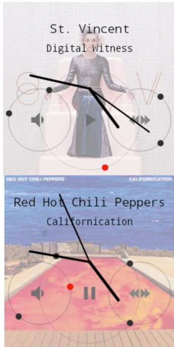
Figure 2: Two examples of the music player application. In this interface, three Orbits enable users to play and pause a song (center Orbit), increase or decrease its volume (left Orbit) and skip back or ahead in the playlist (right Orbit). Both left and right Orbits have two targets moving in opposing directions (clockwise: increases the volume, skips ahead; counterclockwise: decreases the volume, skips back). A red target represents a user selection.
