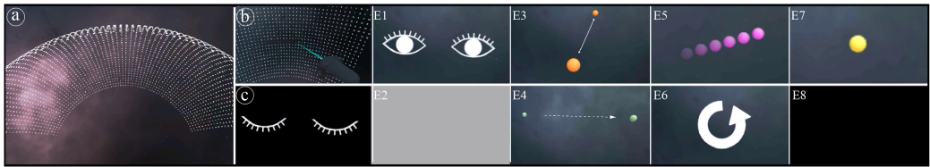
Fig. 8. Screenshots of the custom VR eye exercise application: (a) the WordSearch Puzzle implemented as a hemisphere of letters, (b) point of view of participants during the study task, this was same for the control condition, (c) + E1–E8: instructions for the eye movements (arrows depicted here to indicate animations within the instructions), and closing the eyes, E1 : periodic blinking, E2 : pupillary light reflex (with changing background), E3 : fixation shift, E4 : saccades, E5 : smooth pursuit, E6 : rolling eyeball into one direction, E7 : static fixation, and E8 : loose focus with open eyes. A video of the eye exercises is given in the supplemental material.
