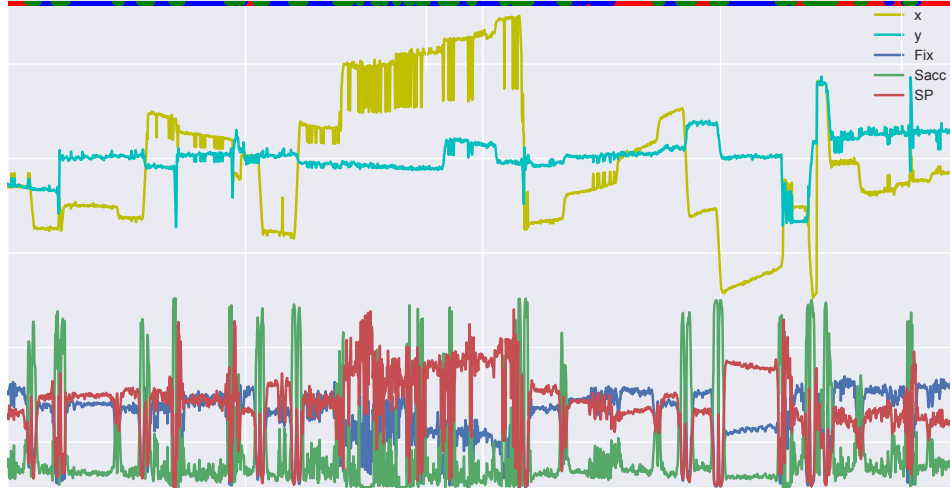
Figure 4: Given the gaze stream on top, the activation is plotted on the lower half of the figure. Each colour of the activation stand for the probability one class of eye movements - i.e. at each time frame, the prediction would be the class corresponding to the highest curve. The colours in the top line indicate ground truth labels.
