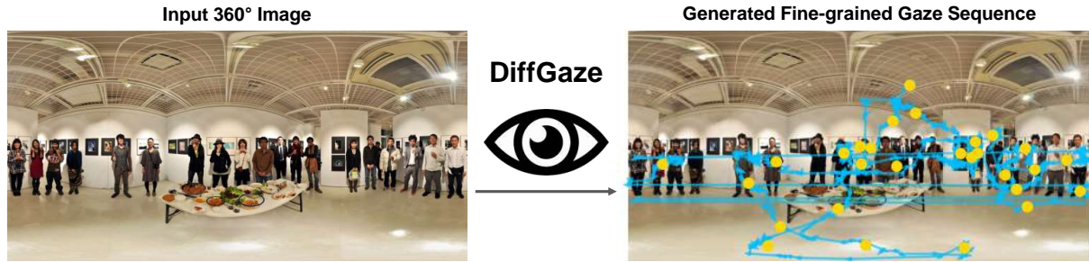
Fig. 1. In stark contrast to scanpath prediction , which only focuses on predicting sequences of fixations (yellow), fine-grained gaze sequence generation is the much more challenging task of faithfully and holistically modelling human gaze behaviour (blue) that resemble the gaze data recorded by eye trackers (normally 30 Hz - 1000 Hz). We present DiffGaze — the first method for fine-grained gaze sequence generation on 360° images. DiffGaze aims to model eye events with very different velocity distributions, e.g. fixations and saccades, formulating the fine-grained gaze sequence generation task as a conditional diffusion process conditioned on the image features.
