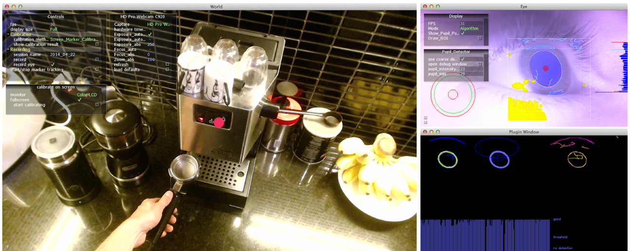
Figure 5. Screen capture of Pupil Capture. World) Window displays real-time video feed of the user’s FOV from the scene camera along with GUI controls for the world camera and plugins. Red circle is the gaze position of the user. Eye) Window displays real-time video feed of the user’s eye from the eye camera with GUI controls for the eye camera and plugins for the eye process. Plugin Window) plugins can also spawn their own windows. Shown here is a plugin to visualize the pupil detection algorithm.
