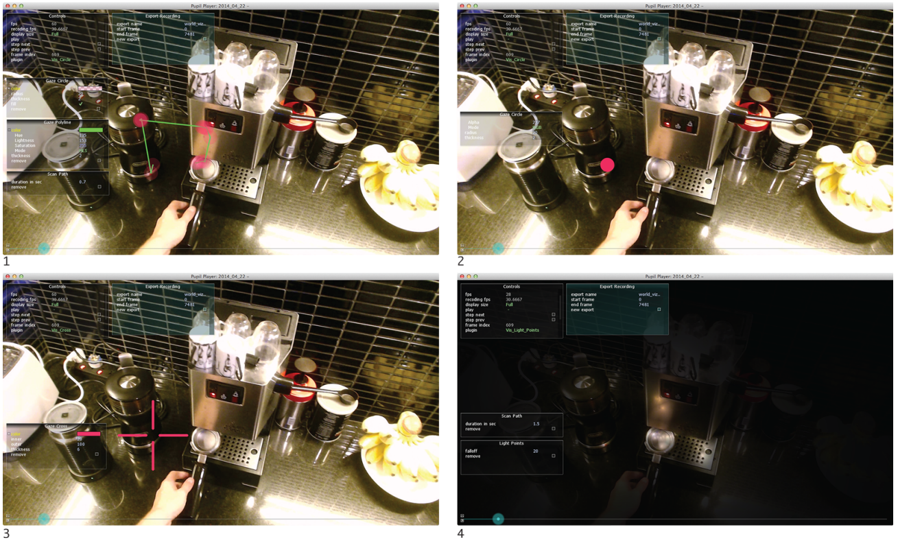
Figure 7. Screen captures of Pupil Player demonstrating four different visualization methods of the same scene at the same point in time. 1) Screen capture of Pupil Player showing a visualization of gaze data and scene video recorded with Pupil Capture. Three plugins used additionally to generate the visualization: i) Scan Path - shows gaze positions within duration set by the user and uses optical flow to compensate for ego-motion. ii) Gaze Circle - translucent red circles drawn for each gaze position within the range set by the Scan Path plugin. iii) Gaze Polyline - green line that connects the gaze positions in temporal order. 2) Gaze Circle visualization current data point as red filled circle. 3) Cross visualization - current data point as red cross mark. 2c) Gaze Polyline - gaze points within temporal duration of Scan Path are shown as green polyline. 4) Light Point Transform - gaze points within temporal duration of Scan Path are shown as white white points
