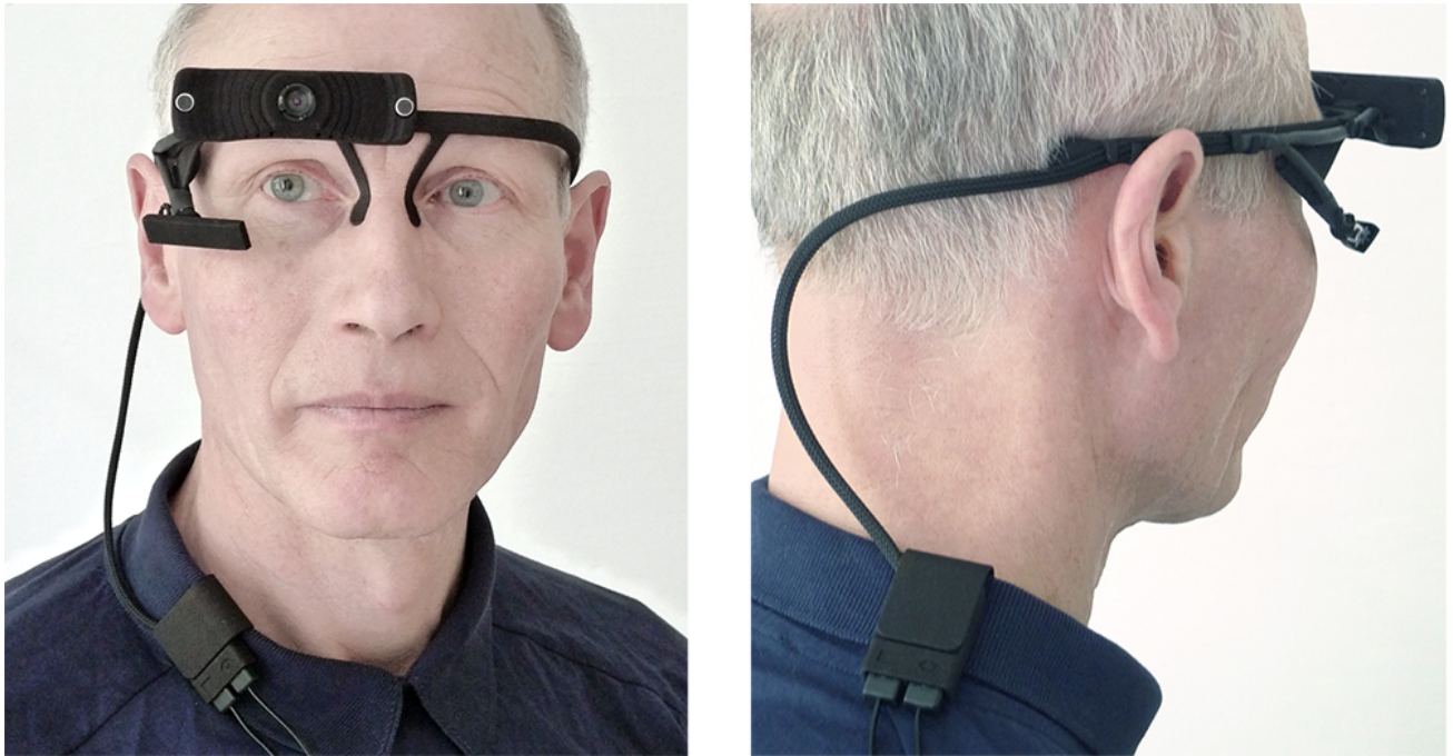
Figure 2. Pupil Pro r021. Front view of Pupil Pro (left image), shown with cable clip attached to user's collar. View from behind right (right image) with rotating clip attachment and flexible cable from headset to cable clip. Clip and lightweight and flexible cable enable greater freedom of head movement.
