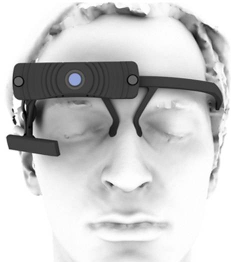
Figure 1. Front rendering of the Pupil Pro headset (rev 20) showing the frame, tilttable scene camera and rotatable eye camera.
