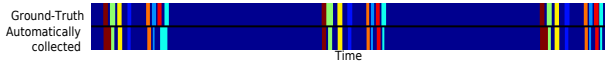
Fig. 4: Labels from offline video-based annotation (top) and automatic annotation from ambient infrastructure (down). There is label boundaries jitter and and some labels do not match.
