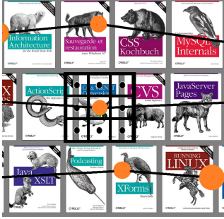
Figure 3: Proposed approach of sampling eight additional image patches around each fixation location to compensate for eye tracker inaccuracy. The size of orange dots corresponds to the fixation’s duration.
