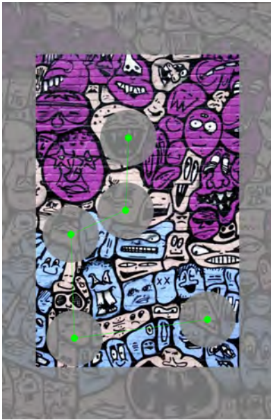
Figure 3. When defining a password on an image, SmudgeSafe allows the user to select password points from a central area of the image. This is to ensure that transformations significantly change password point locations while preserving a reasonably large theoretical password space.
