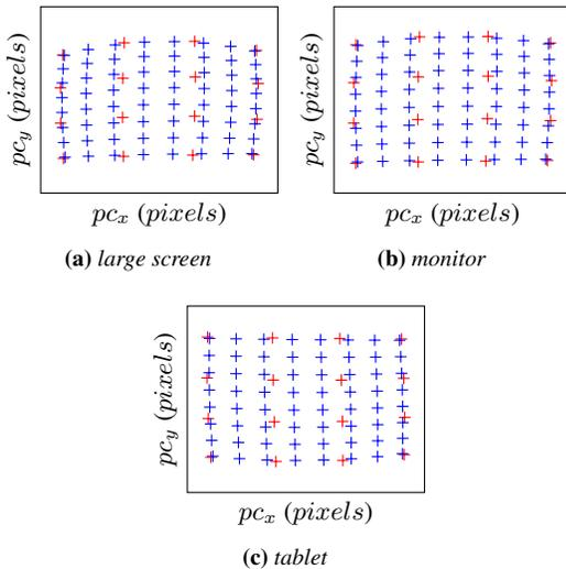
**Figure 2:** Pupil center coordinates when looking at the calibration points (red) and test points (blue).
