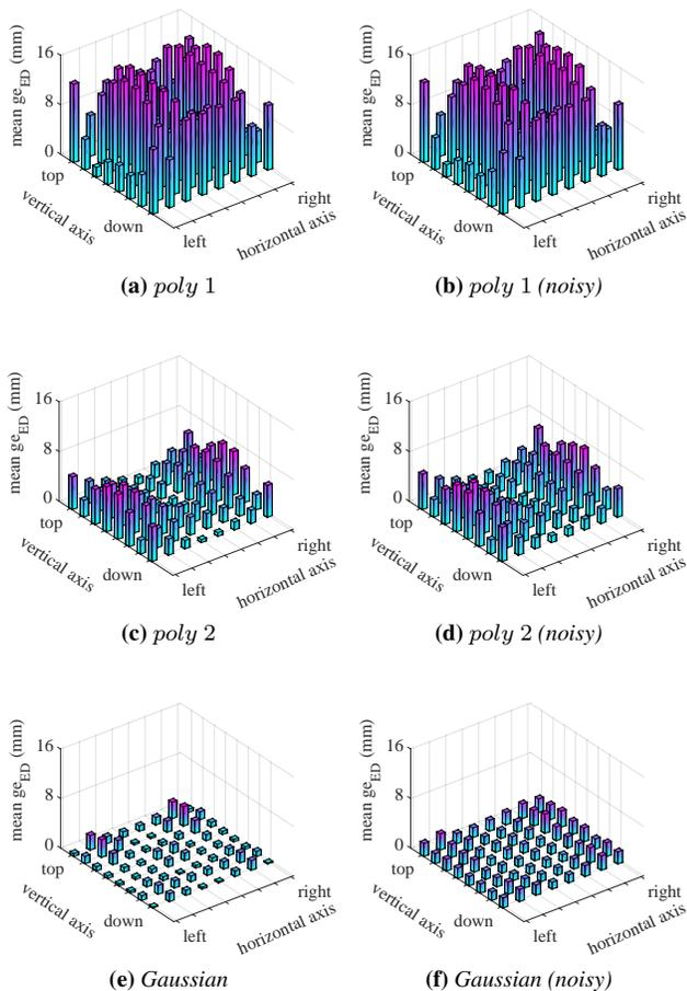
**Figure 3:** Euclidean gaze estimation error in mm for a simulated user for the test grid for a large screen and camera focal length 35 mm when using three different regression functions with the normalized pc-cr vector with perfect feature detector's and with Gaussian noise with zero mean and std 0.1 pixels.
