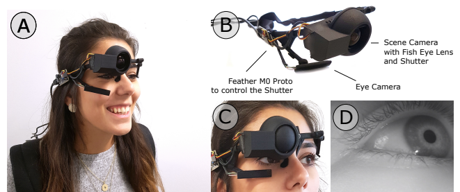
Figure 2: PrivacEye prototype with labelled components (B) and worn by a user with a USB-connected laptop in a backpack (A). Detection of privacy-sensitive situations using computer vision closes the camera shutter (C), which is reopened based on a change in the privacy detected level in a user’s eye movements (D).
