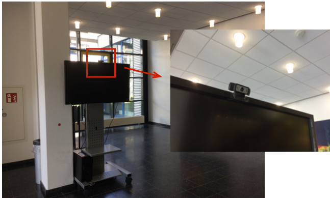
Figure 5: We deployed AggreGaze in a public space for two weeks. The recording setup consisted of iiyama ProLite 46-inch display, a Logitech C930e webcam, and a host computer running our custom recording software.
