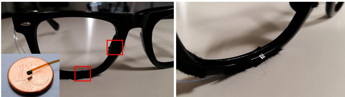
Fig. 2. Fully integrated version of *InvisibleEye* consisting of multiple, millimetre-size Awiba NanEye RGB cameras (marked in red) that are invisibly integrated into an off-the-shelf glasses frame. For our evaluations we developed two other prototypes to be able to characterise performance across key design parameters, including image resolution and number of cameras, as well as camera angle and positioning, and to compare with a state-of-the-art (high-resolution) mobile eye tracker.
