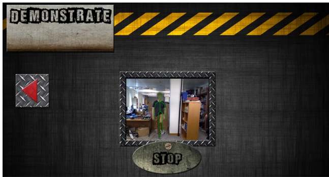
Figure 7: Demonstration interface. The user can see his skeleton overlaid on top of the colour image recorded by the Kinect. The recording is controlled by voice commands.
