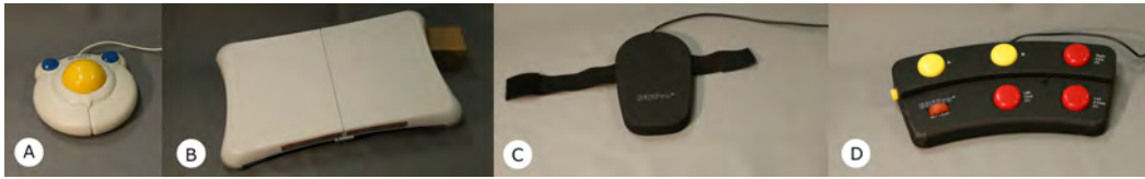
Fig. 2: Mediated sensing using computer peripherals: (A) large trackball [Pakkanen and Raisamo 2004]; (B) Nintendo Wii Balance Board [Daiber et al. 2009]; (C,D) BiliPro Foot Mouse and Keys
