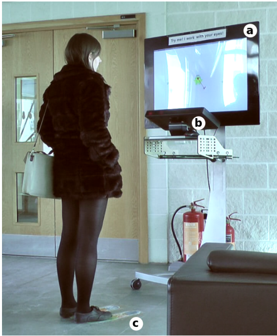
Figure 12: The setup of the field study. (a) Screen with frog game. (b) Eye tracker. (c) Placement footmarks with colours depending on the user's height. The field study showed that users were able to interact without given assistance.
